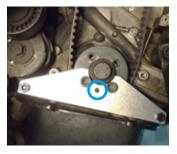
Tighten the belt to the maximum value of the tensioner and tighten the fixation of the tensioner.
