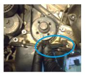
Turn crankshaft carefully to be able to place the tool (1860901000) so that the hole of the tool matches the pinion pin.
