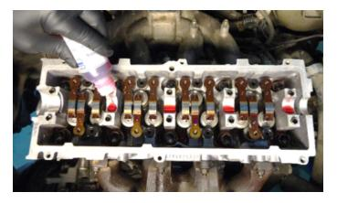
Before positioning the new camshaft, ensure that there is not any of the pistons at Top Dead Center (TDC) to prevent valve shock during the camshaft bearings tightening.
